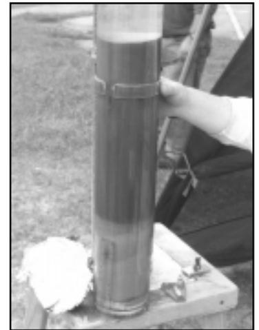
**Sediment Core from Crystal Lake (2201). Note the unusual lighter sand layer below the darker marl lower indicating the 1873 draw down event.**
